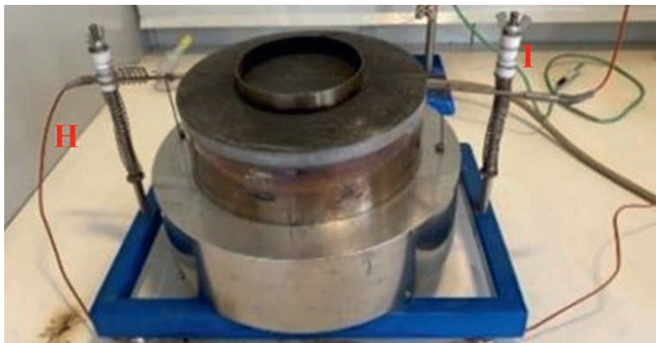
Fig. 2. Hot-plate device; H – thermocouple in the plate for temperature recording, I – thermocouple for temperature recording in the layer of dust (Photo. J. Jađuřová)
